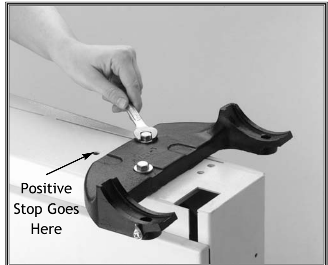
Figure 17. Attaching trunnion support to body.
